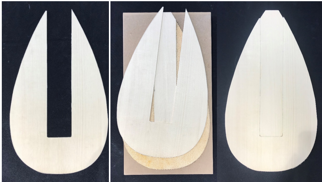
Image 4, 5, and 6. Preparations of the second soundboard for the sandwich table
