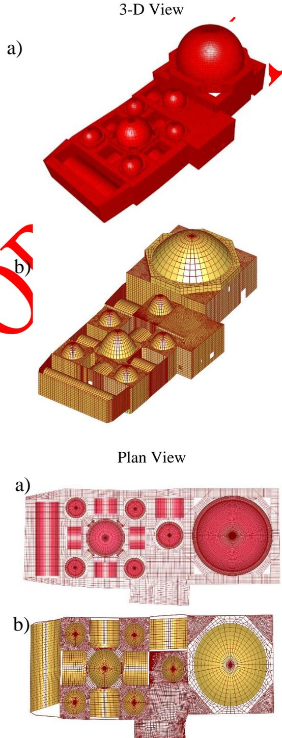
Figure 6. a) Solid model b) Shell model
