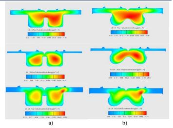
Fig.11. Distribution of TKE in cylinder's central plane. a) Piston A (standard piston) b) Piston B
