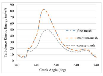
Fig. 3. TKE for different mesh densities
