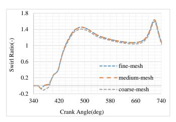
Fig. 2. Swirl ratio for different mesh densities
