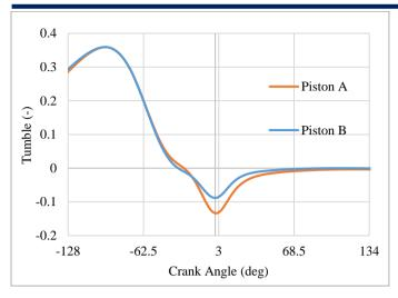
Fig.9. Tumble ratio for piston bowls
