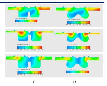
Fig.7. Distribution of velocity in cylinder's central plane a) Piston A (standard piston) b) Piston B
