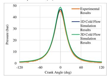
Fig. 5. In-cylinder pressure curves for cold flow
