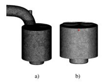
Fig. 4. Computational grid a) intake stroke b) closed part of the cycle.
