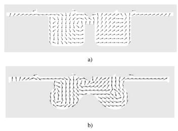
Fig. 8. Distribution of velocity vectors in cylinder's central plane at TDC. a) Piston A (standard piston) b) Piston B
