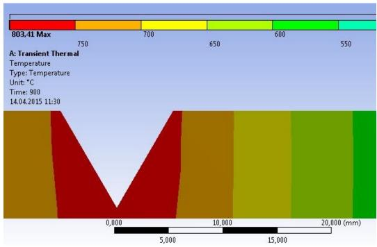
Figure 3. Temperature gradient formed into HAZ
