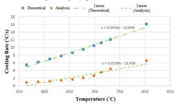
Figure 4. Comparison of theoretical and analysis cooling rates
