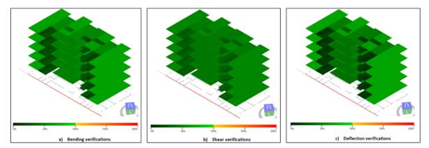
Figure 14. Verification percentage of floors, a) and b) Ultimate Limit State (ULS), c) Serviceability Limit State (SLS)
