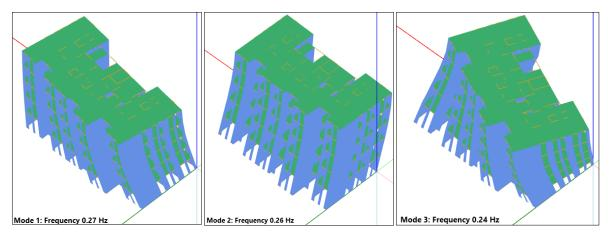
Figure 10. The first three mode shapes
