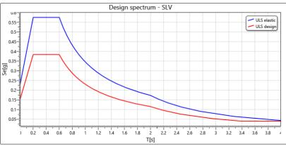
Figure 8. Design spectrum according to Eurocode
