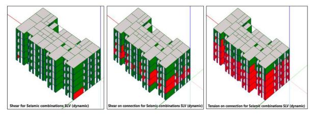
Figure 13. Shear and tension failures in the elements and connections of the model for SLV (Life safety limit state, dynamic)
