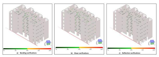
Figure 15. Verification percentage of beams, a) and b) Ultimate Limit State (ULS), c) Serviceability Limit State (SLS)
