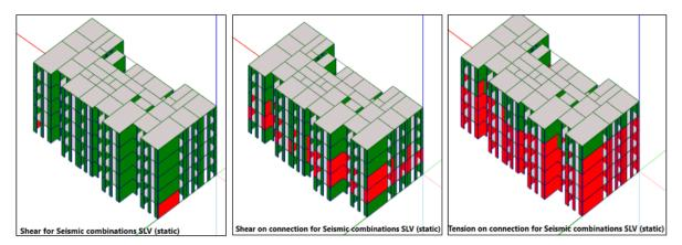
Figure 12. Shear and tension failures in the elements and connections of the model for SLV (Life safety limit state, static)
