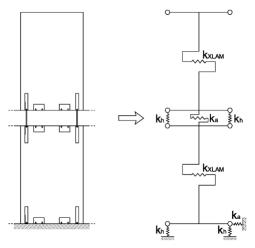
Figure 6. Total stiffness of CLT walls
