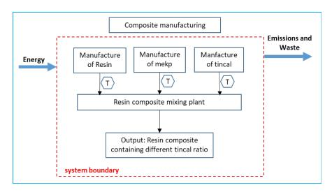
Figure 5: The system boundary of tincal reinforced resin composite production (T: transport).
