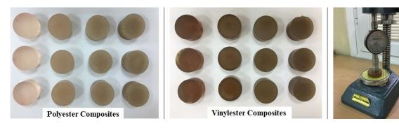
Figure 3: Shore D hardness testing of polyester and vinylester composites.
