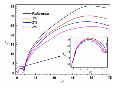
**Figure 10:** Cole-Cole diagram of tincal reinforced vinylester composites.
