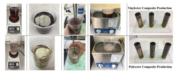
**Figure 1:** Preparation of tincal-reinforced vinylester and polyester composites.
