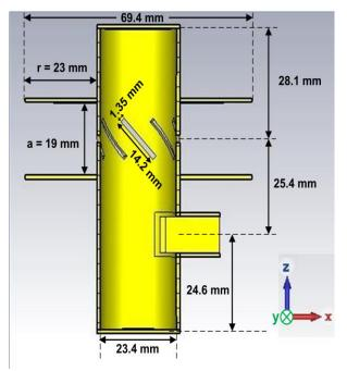
Figure 11. The dimensions of the designed antenna with identical slots for telemetry purpose (transmitter structure).
