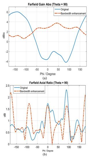
**Figure 15.** (a) Rectangular radiation patterns and (b) axial ratio of the antennas of first and second versions in azimuth plane at 12.25 GHz.
