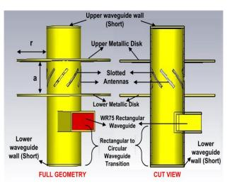
**Figure 4.** The proposed circularly polarized omnidirectional antenna structure along with cut view for both versions.
