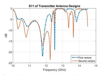
**Figure 12.** The magnitude of reflection coefficient  $(S_{11})$  of the designed transmitter (telemetry) antennas.
