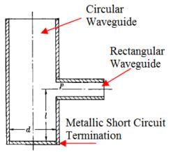
Figure 1. Rectangular-to-circular waveguide structure [20].
