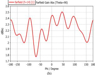
**Figure 8.** Simulated (a) polar radiation patterns and (b) rectangular gain pattern at the azimuth plane for receiver (telecommand) antenna at 14 GHz.
