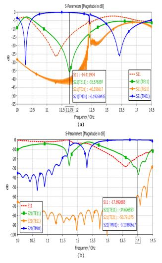
**Figure 3.** The magnitudes of S-parameters (reflection and transmission coefficients) of the designed transitions for (a) transmitter structure (b) receiver structure.
