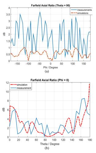
**Figure 10.** The rectangular axial ratio patterns (a) for azimuth plane (b) for elevation plane.
