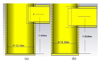
**Figure 2.** Final dimensions belonging to designed rectangular-to circular waveguide transition (a) for transmitter structure (b) for receiver structure.
