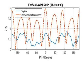
Figure 14. The axial ratio patterns of the antennas of first and second versions in azimuth plane at 11.75 GHz.
