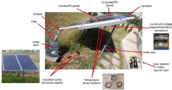
**Figure 3.** Experimental setup and designed cooling system.
