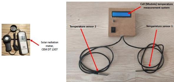
**Figure 5.** Solar radiation measurement and temperature measurement devices.
