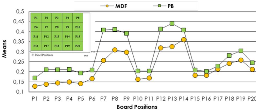
Figure 3. Impact of the different board positions on measurements (MDF and PB)
