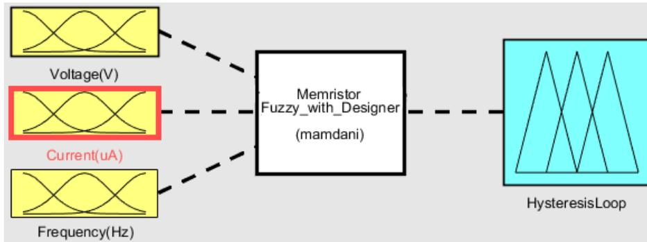
Figure 3. Fuzzy logic-based memristor hysteresis assessment model.
