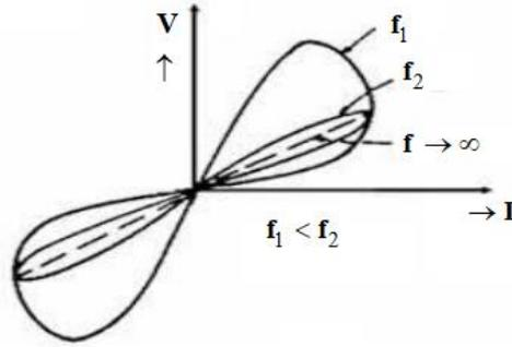
Figure 1. Hysteresis curve of memristor (Wen et al., 2018).
