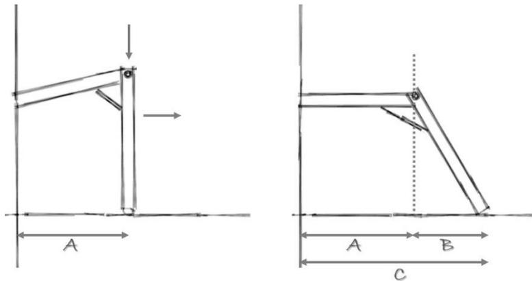
**Figure 13.** Abstracted movement mechanism (closed - open) [21]
